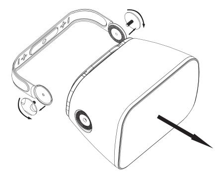
Next install the speaker mounting bracket firmly to the mounting surface using the supplied mounting hardware.
