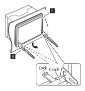
2 When the lower level is removed, remove from the upper two catches of the trim plate (6).
