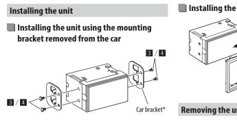
Note: Select the appropriate screws (supplied) for the mounting bracket.
