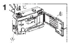
Press the talon (A) in the direction of the anow and open the camera tack coor (B) Lift up the film rewind mark (C) and place at new ratiof from into the film chamber.
