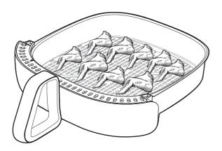
4. Insert the basket with the handle into the Air Fryer securely. The Air Fryer will not start cooking if the basket is not securely inserted. If this happens, the temperature and time display will show "---" and "--", respectively.
