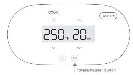
8. Press the "**Start/Pause**" button to temporarily pause the cooking process. (The temperature and time settings can be adjusted during cooking)
