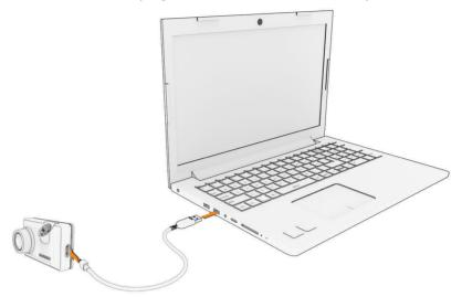
2 Plug the other end of the cable into a compatible USB port on your computer.
