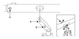
Align Optical Tube (OTA) Mounting Brackets with holes (A) on top of Alt-Az Mount Arms and secure with Mount Knobs (B). When attaching optic to mount, make sure Threaded Holes on OTA (C) and Mount (D) are facing you to complete step 6.
