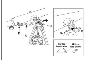
6. Slide Altitude Rod (A) through hole (B) on Vertical Adjustment Knob located on Alt-Az Mount Arm. Secure with Vertical Adjustment Knob (C). Use the included Slotted Screwdriver to secure Altitude Rod to the OTA Threaded Hole (D) with Altitude Rod Screw.
