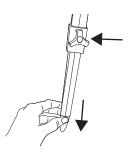
Pull legs down to desired height. Insert a **Tripod Leg Knob** into each of the 3 tripod legs and tighten.
