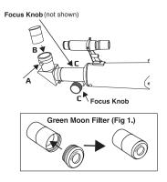
Loosen thumbscrew (A) on erecting diagonal. Slide H20 Eyepiece\* (B) into erecting diagonal and tighten thumbscrew (A) to secure. Adjust Focus Knobs (C) on OTA until image is clear. IMPORTANT: Erecting diagonal must be used with eyepiece.
