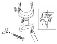
Remove Wing Nuts from Leg Screws. Align holes on top of Tripod Legs on Alt-Az Mount Base. Insert Leg Screws into each of the 3 legs and base. Secure with wing nuts.
