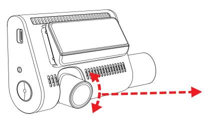
Rotate front dash cam lens so that it is parallel with the road.
