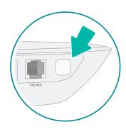
Pair Linx with Telo by pressing the Page button on the Telo for 3 seconds
