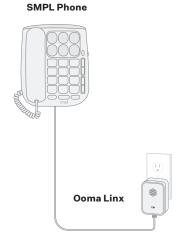
**b-4**Telo, modem/router, SMPL phone, and Linx setup
