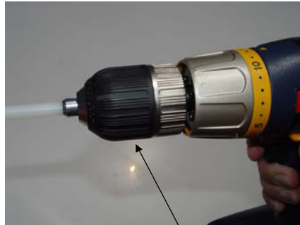
Twist chuck to tighten
