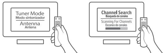
In the TV's setup menu, set the tuner mode to "Antenna" or "Air". Then, set the TV to "scan" for channels. This may be listed as auto-program, auto-scan, channel search, or channel scan. Refer to the TV manual for detailed instructions.
