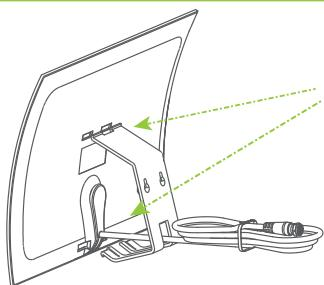
FIRST, insert the top of the antenna stand into the slots at the top of the antenna, THEN insert the bottom of the stand into the double slots at the bottom of the antenna.
