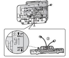
Insert the lower tabs of the adaptor into the unit's bottom slots (1), then insert by pushing down the levers of the adaptor into the upper slots (2).
